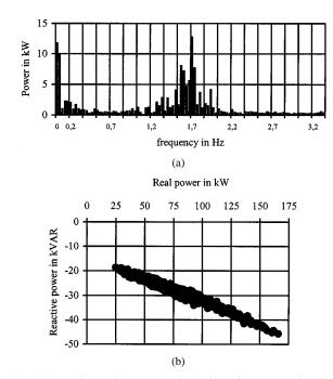
Fig. 1. (a) Power harmonic spectrum. (b) Real/reactive power ratios.
