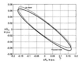
Fig. 7. Comparative results of power fluctuations between third-order dynamic model and proposed model  $P_{nt,0} = -0.992$  p.u.,  $Q_{nt,0} = 0.2786$  p.u.
